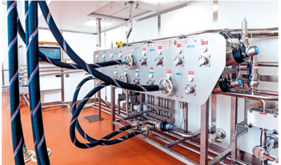
The Turck BL ident system reliably prevents incorrect coupling and thus ensures consistent product quality
