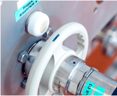
As soon as the hose is connected, the RFID system verifies the connection
